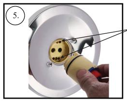
Align pins with cartridge and valve body when reinstalling cartridge
